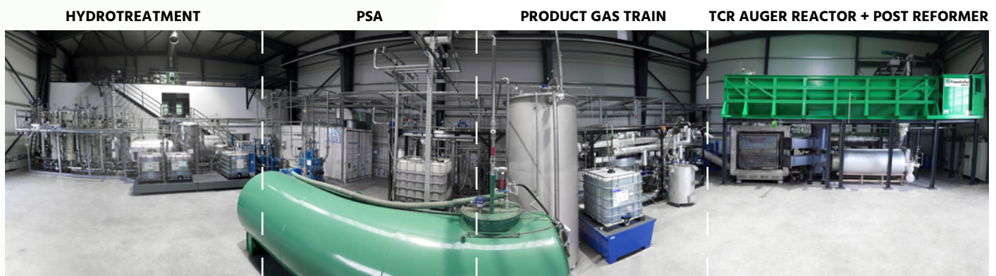
Figure 5: Complete process chain of TO-SYN-FUEL-demonstrator. Credit: Fraunhofer UMSICHT.
